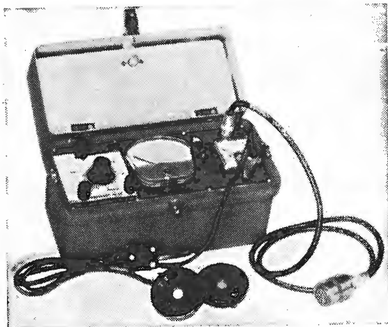
Dawe 1103 thickness gauge, showing the transducer.
